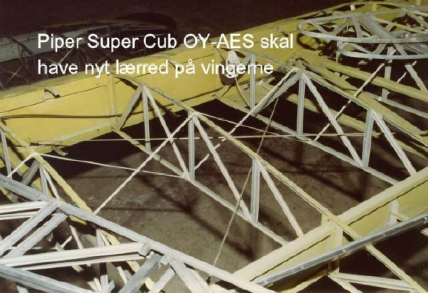
A close-up, low-angle photograph showing the intricate internal truss structure of an aircraft wing. The structure is composed of numerous light-colored, metallic beams forming a complex network of triangles. The wing itself is painted a bright yellow color. The background is dark, making the yellow paint stand out.
